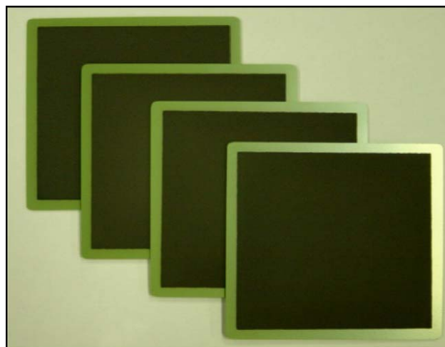
Fig. 1. Photograph of anode-supported 10 cm × 10 cm unit cells.
